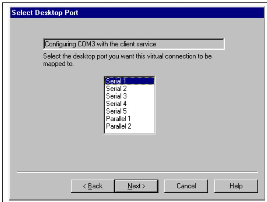
Since the desktop port is Serial 1, the label printer can be attached to a ThinSTAR. The ThinSTAR 500.NET models have one serial port and one parallel port.
