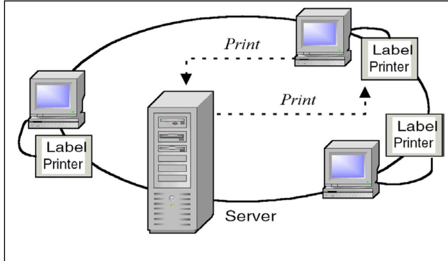
In both of these cases, a serial or parallel device port is mapped to a virtual port on the server using the Use Client Service option (rather than the Use Specified Client Hostname option). The following example shows a completed port assignment for label printers. The Port Option column shows the selected settings.
