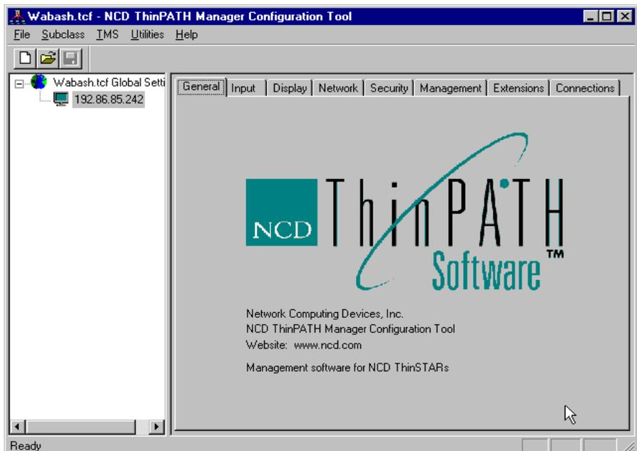
This tool shows the same allowable settings in the same locations as in Terminal Properties. Parameters that cannot be set globally, such as a static IP address, however, are not included in the NCD ThinPATH Configuration Tool. Other parameters are available only through the NCD ThinPATH Configuration Tool. These are described in *Relationship to NCD ThinSTAR Terminal Properties* on page 6.
